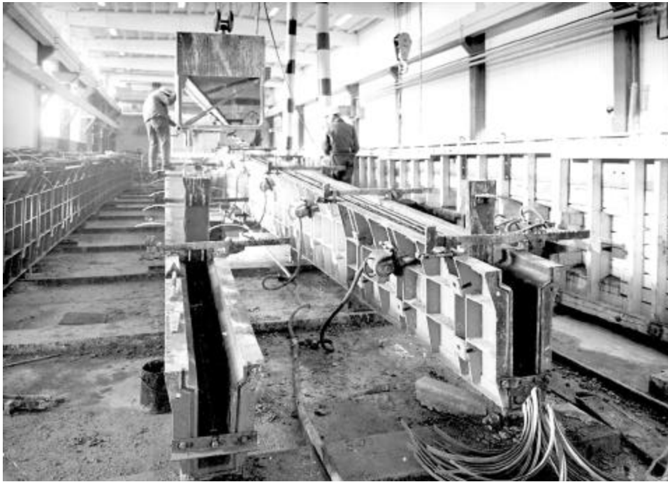
Fig. 12.4—Form vibration used in precast beam construction
