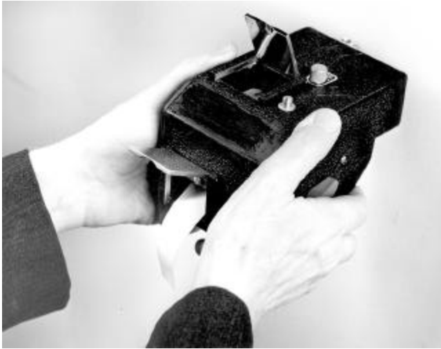
Fig. 15.3.3—Using vibrograph to determine amplitude and frequency of vibrating form
