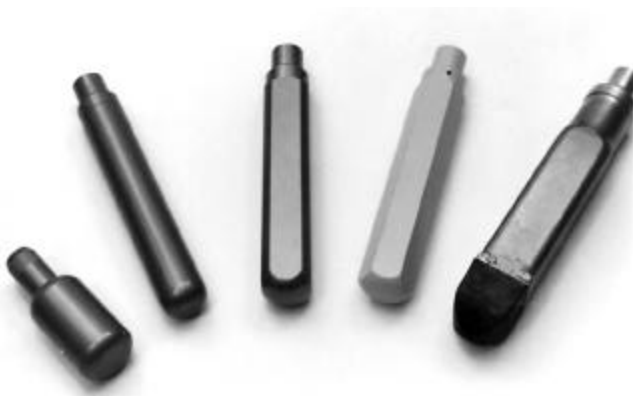
Fig. 5.1.6—Several of the different sizes and shapes of vibrator heads available. From left to right: short head, round head, square head, hexagonal head, and rubber-tipped head
