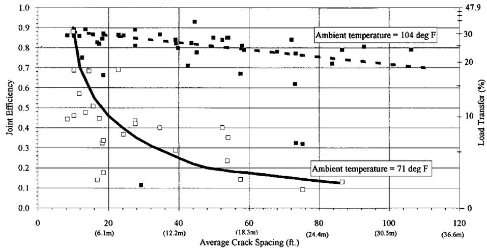
Fig. 9.7.3—Relationship between joint efficiency, load transfer, and average crack spacing, Ft. Drum, New York
