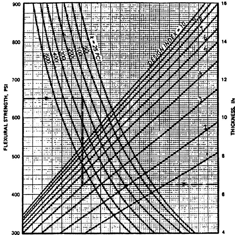
Fig. 6.2.2—Corps of Engineers design chart for RCC pavements
