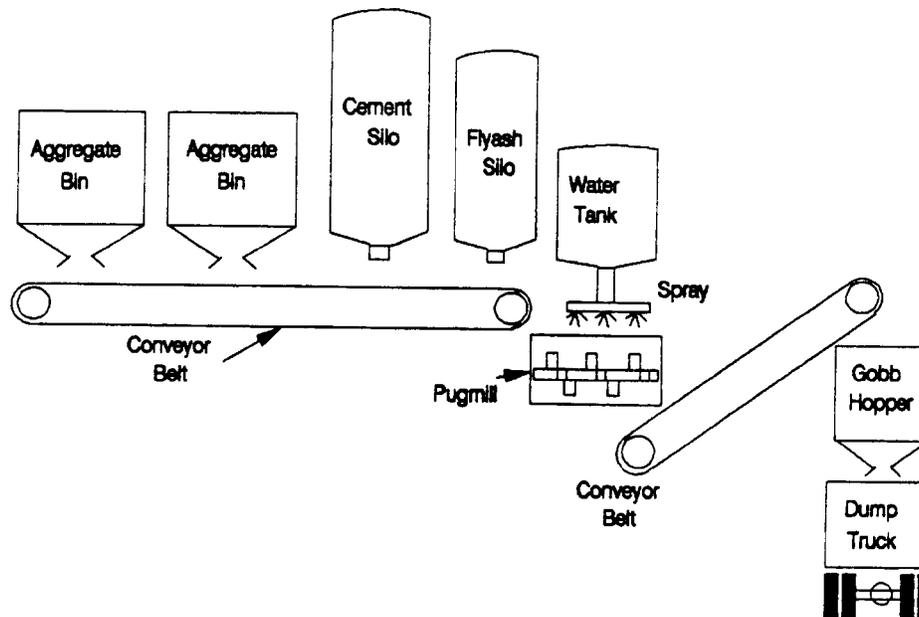
Fig. 7.3—Schematic of continuous mixing pugmill plant
