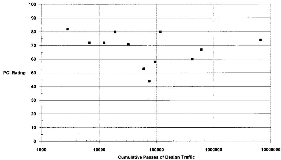
Fig. 9.2.2—Variation in PCI with cumulative passes of traffic
