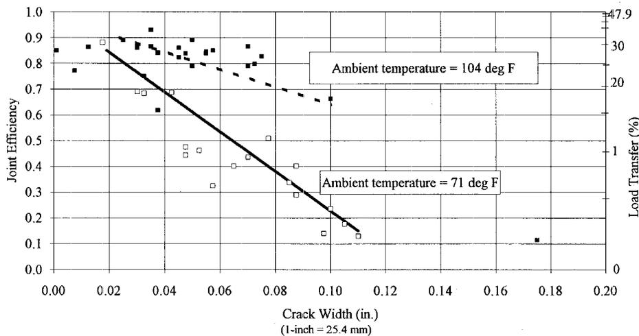
Fig. 9.7.4—Relationship between joint efficiency, load transfer, and crack width, Ft. Drum, New York
