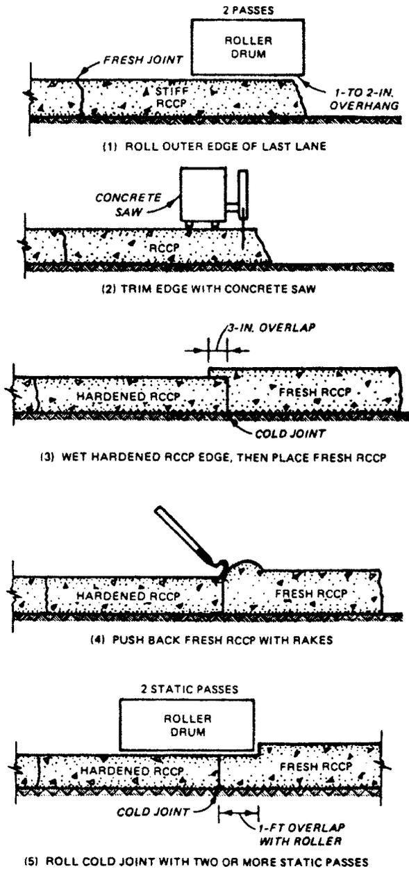
Fig. 7.6.2—Roller pattern for cold construction<sup>16</sup>
