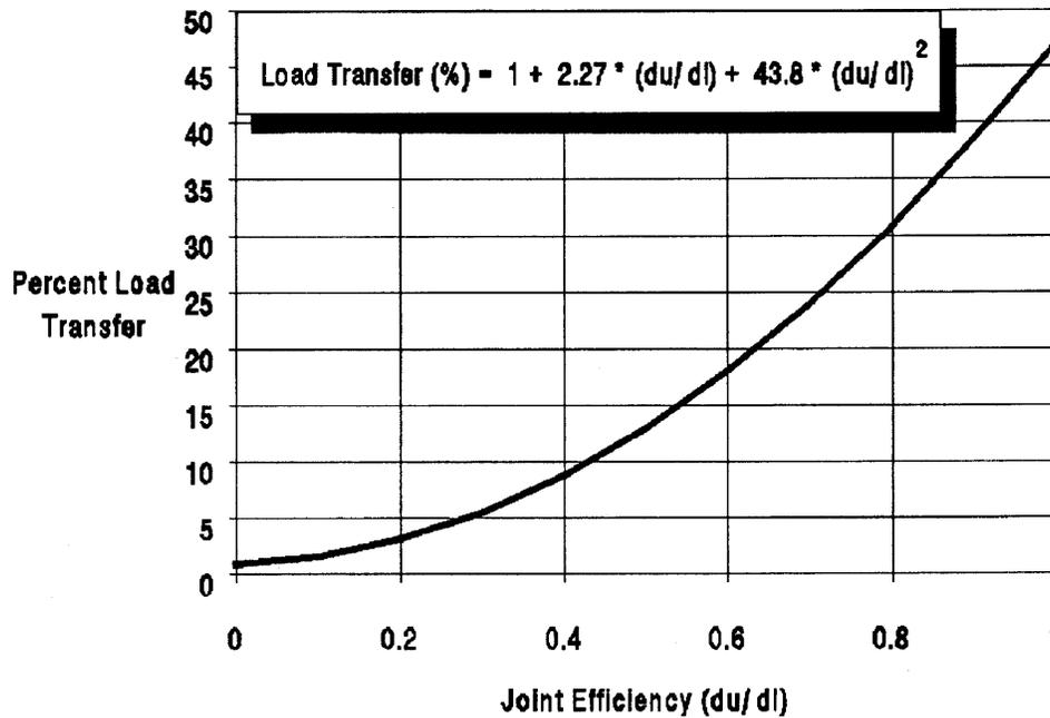
Fig. 9.7.2—Corps of Engineers relationship between joint efficiency and load transfer
