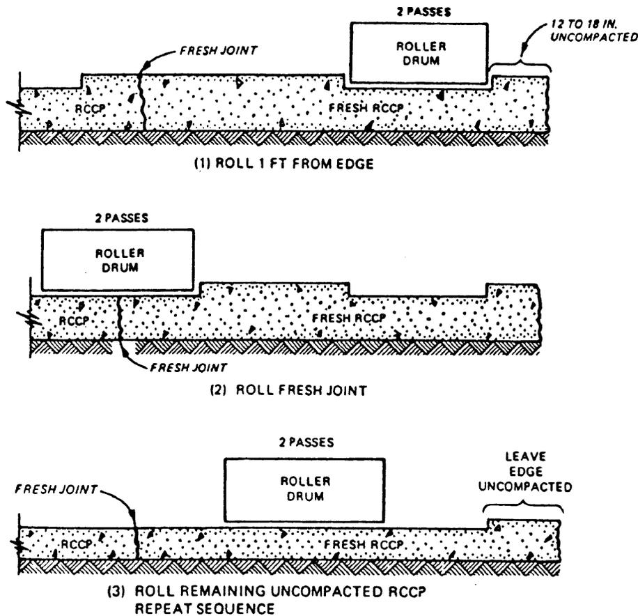
Fig. 7.6.1—Roller pattern for fresh construction joint<sup>16</sup>
