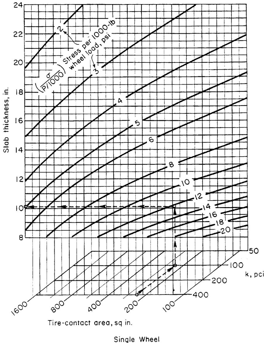
Fig. 6.2.1—PCA design chart for single wheel loads
