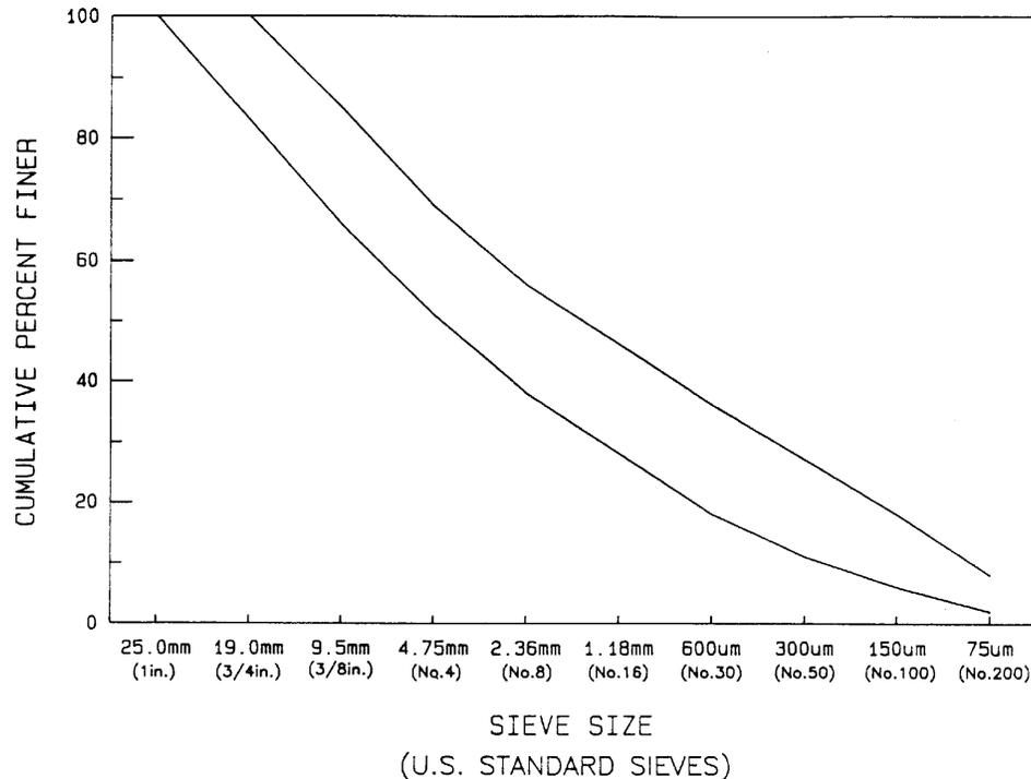
Fig. 3.2—Typical range of RCC pavement aggregate gradation
