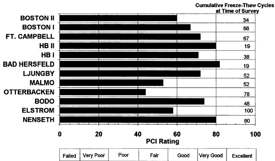
Fig. 9.2.1—PCI rating and estimated cumulative freeze-thaw cycles at time of survey
