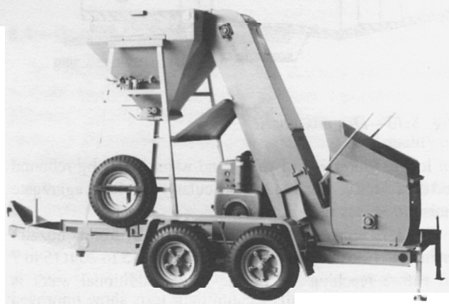
Fig. 3.11a-Batch mixer with elevator for double chamber gun
