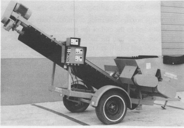
Fig. 3.12-Continuous proportioning mixer with screw elevator has three bins for fine and coarse aggregate and cement
