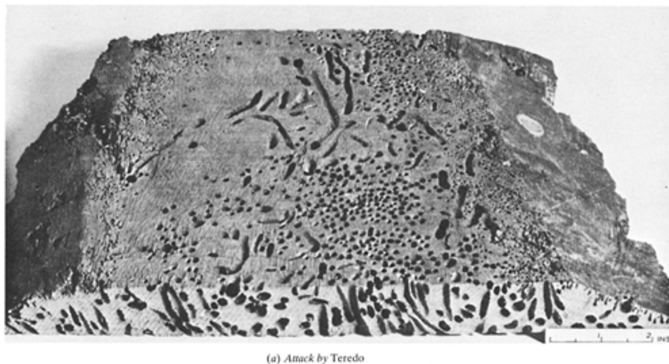
Fig. 10.2 Attack on timber piles by marine borers (Crown copyright reproduced with permission of BRE, Princes Risborough Laboratory)
