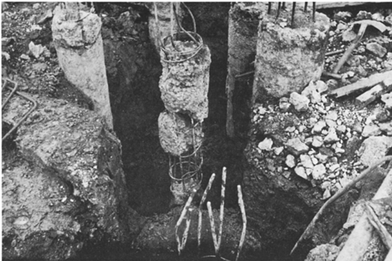
Fig. 3.39 Defective shaft of bored pile caused by cement being washed out of unset concrete
