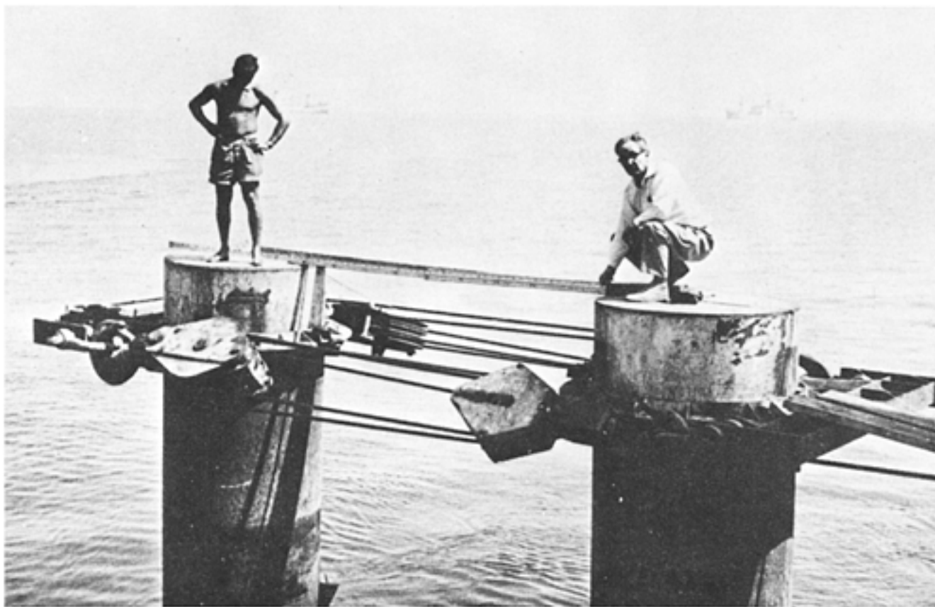
Fig. 11.18 Lateral loading test on two steel tubular piles forming part of breasting dolphin
