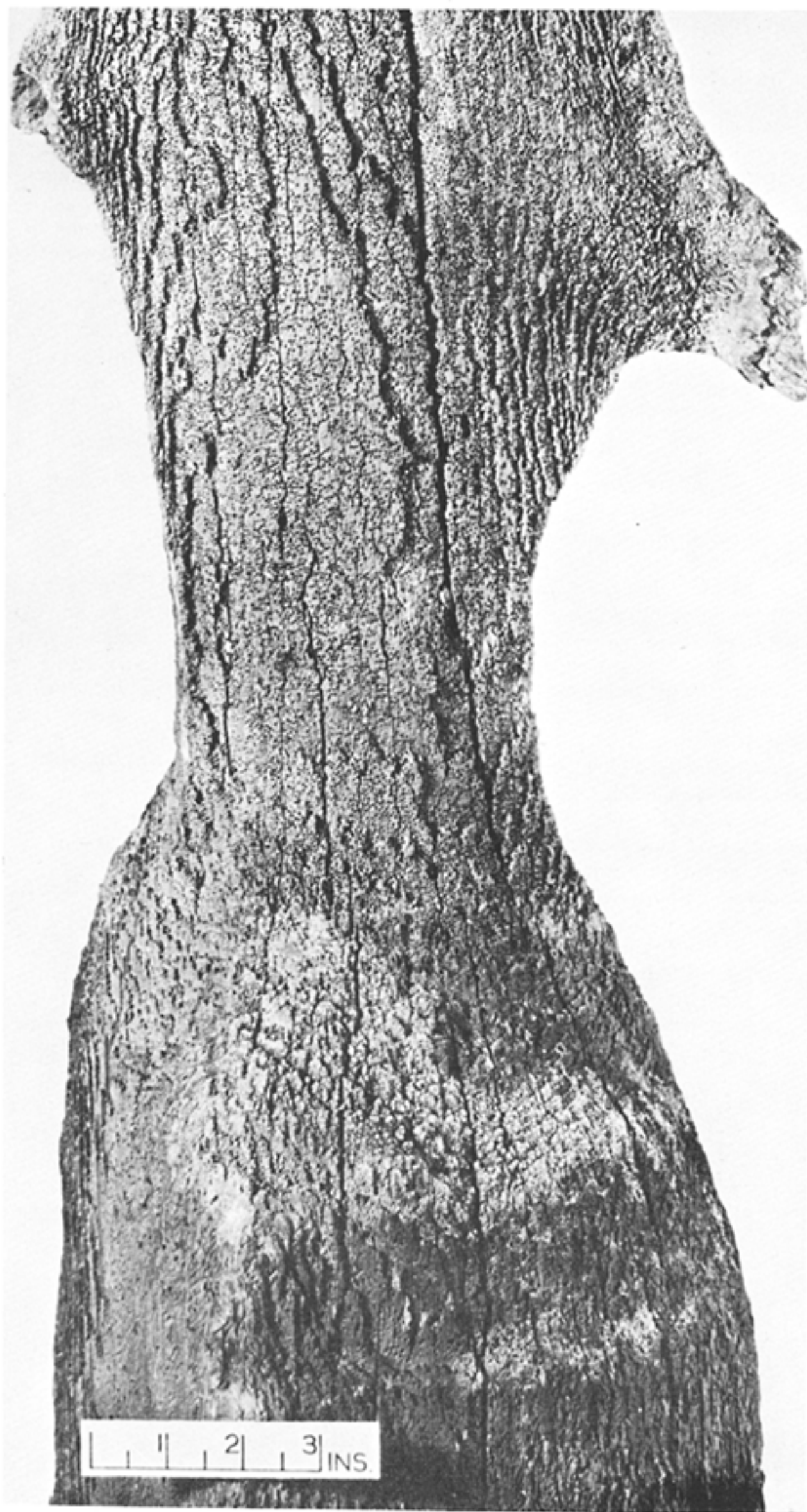
Fig. 10.2 (b) Attack by limnoria (Crown copyright reproduced with permission of BRE, Princes Risborough Laboratory)
