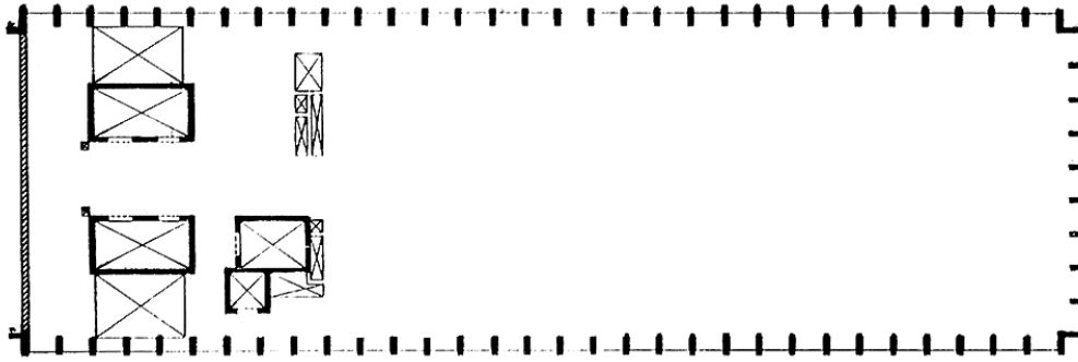
Figure 6-10. False symmetry: offset structural core
