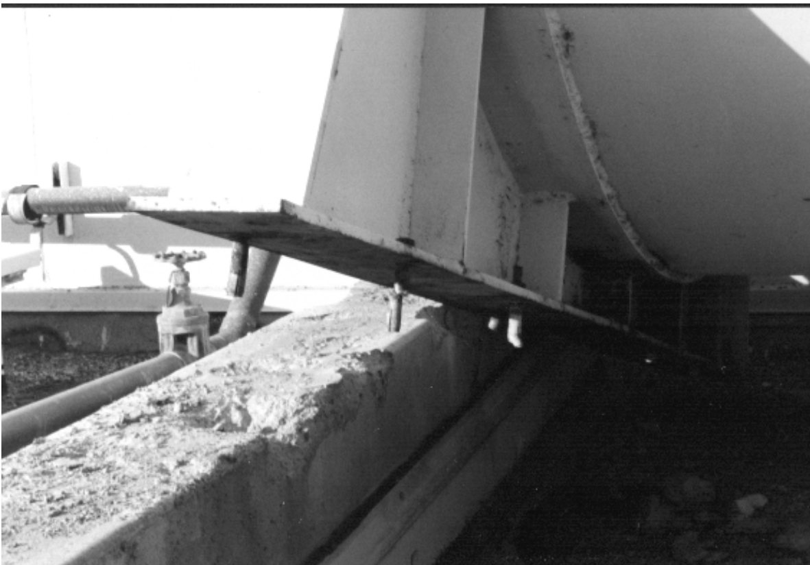
Figure 13-16. Tank in figure 13-2, expansion anchor failure
